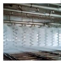
Diffusers from BMA are known around the globe for their outstanding performance and extremely low operating and maintenance costs. With capacities of up to 24,000/33,200 TCD (sugar cane/bagasse), they are extremely flexible and can be tailored to your requirements.
