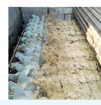
The diffuser from BMA is a fully enclosed, stand-alone horizontal chain conveyor with a rectangular cross section. Its top cover is designed as a rounded steam dome; a special base facilitates the juice flow.
