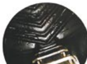
Photos showing vertical movement of cooling water tubes at massecuite surface prior to cooling (reduced level)
