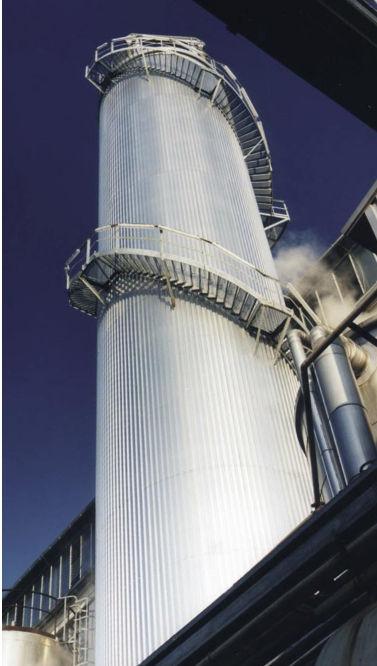
Cooling crystallizer with 600 m 3 net volume
