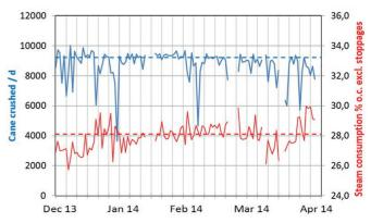
**Figure 6:** Daily crushing capacity and specific steam consumption at ICPL (Step 2)
