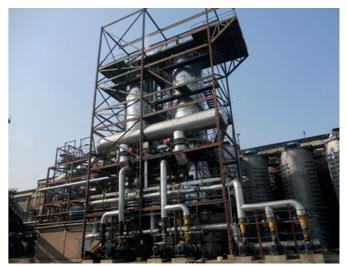
Figure 7: New falling-film evaporators for effect 1 at GSM
