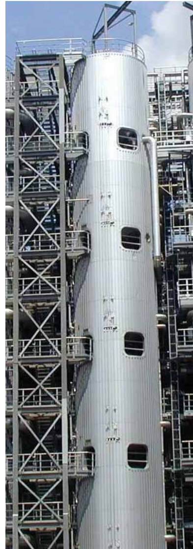
VKT from BMA for continuous crystallisation
