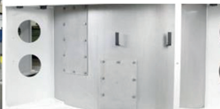
Figure 11: Batch centrifugal: (left) grease collector tray, (right) inspection openings
