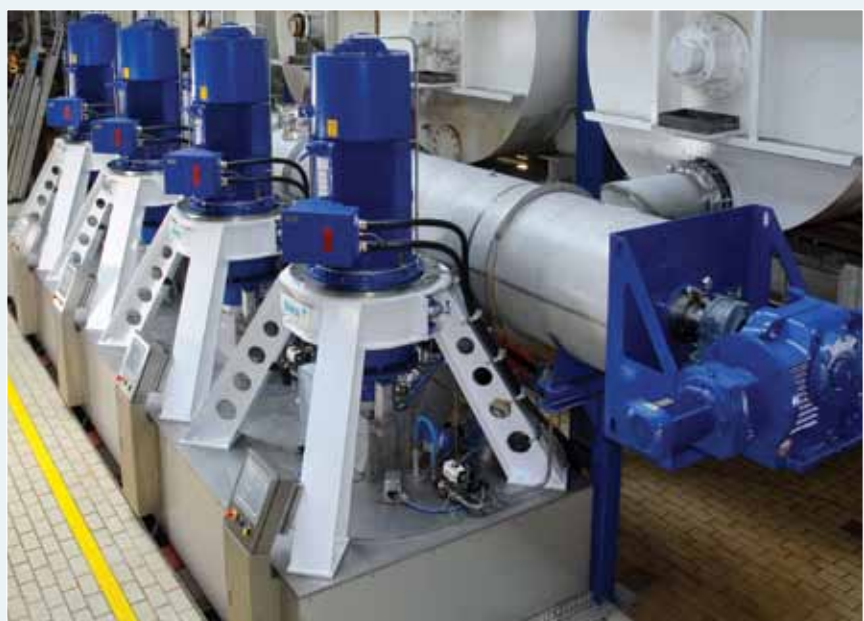
Figure 4. Centrifugal station (in Plattling) equipped with four E1810 centrifugals and a BMA distribution mixer
