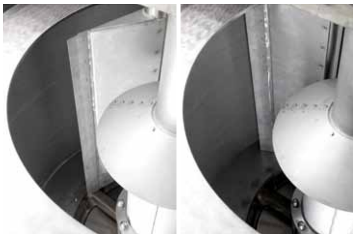
Figure 1. Monaxial discharger in its rest position (left) and swung into its discharging position (right)
