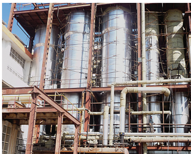
Figure 4: Falling-film evaporators at ICPL / India (3x 4000 m 2 and 2x 1000 m 2 )
