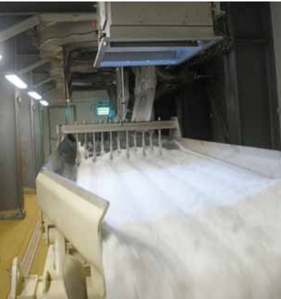
Colorimetric system installed above a vibrating conveyor
