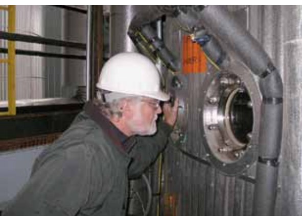
Chris Rhoten checking the massecuite in the 4th chamber of the VKT
