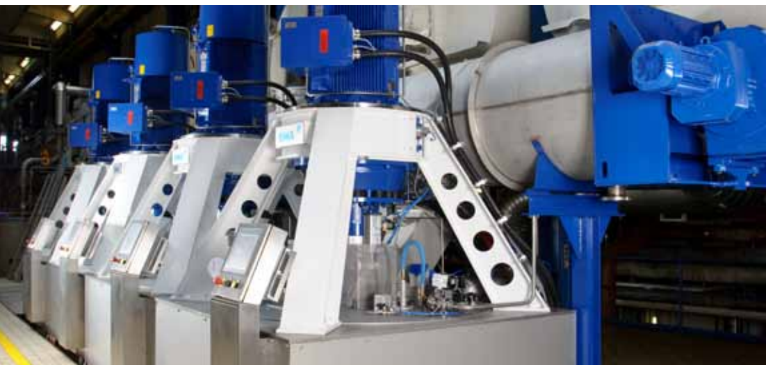
Centrifugal station with new E1810 machines at Südzucker's Plattling plant
