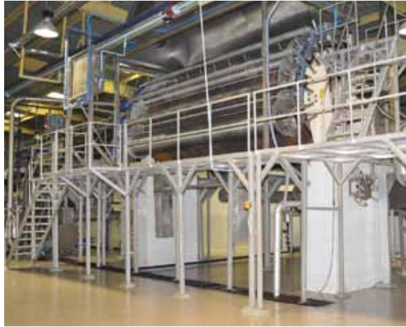
Drum dryer for 500 kg/h of potato flakes
