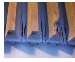
Visual inspection of the bottom-end bearing of the extraction tower
