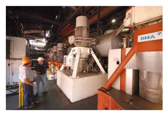
New high-performance B1750 centrifugal at La Unión (on the right: the previous G1750 model)
