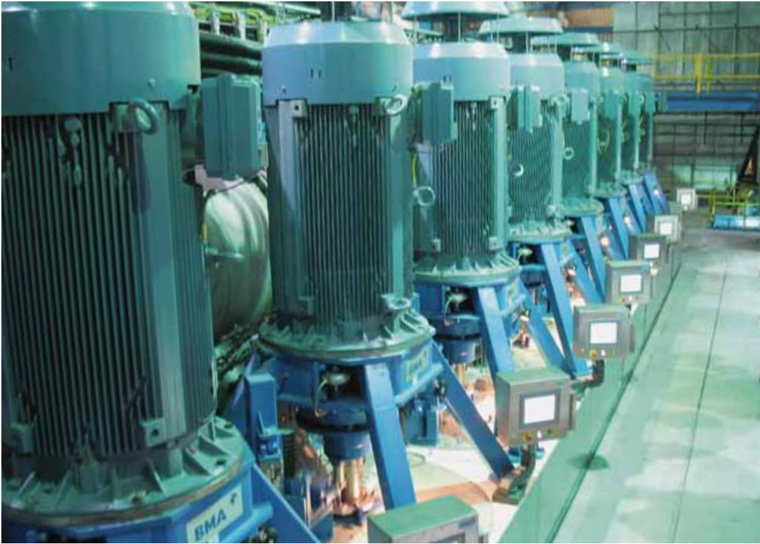
Commissioning of the world's largest centrifugal station for refined sugar (14x B2200-R)
